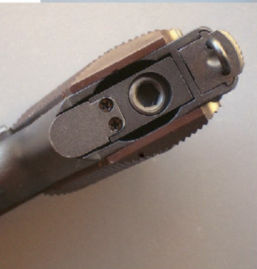
Above: CO2-powered blowback system of Gletcher CLT 1911 provides added realism. Recoil is comparable to a small-caliber pistol. Slide locks open after last shot.
