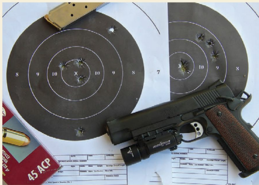
To test the Pro Model with and without a light, left group was shot with light mounted and right without. Although this group shows two shots were "thrown" a bit, other groups with light mounted were as tight as without.
