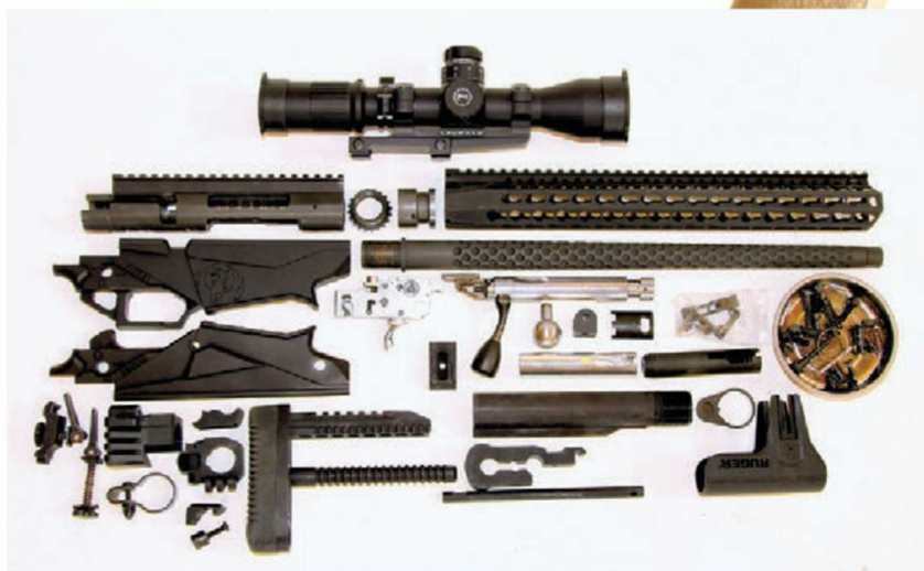
Ruger Precision Rifle completely disassembled and ready to be finished in two shades of Flat Dark Earth Cerakote.
