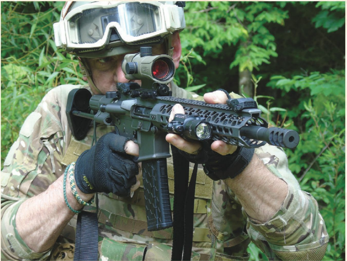
Combination of a 14.5-inch free-floated heavy barrel and a lightweight KeyMod forearm yields a package that is accurate while remaining both maneuverable and easy to hump.
