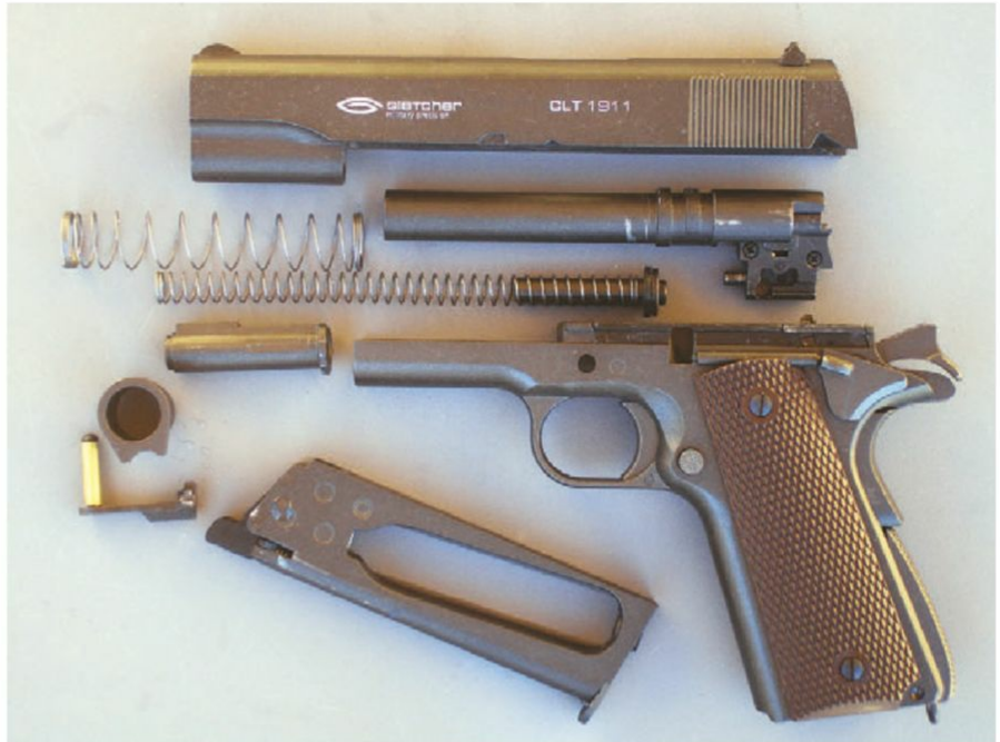
Gletcher CLT 1911 fieldstrips in nearly identical manner to actual M1911. Only difference is that recoil spring plug must be removed from inside the slide.
