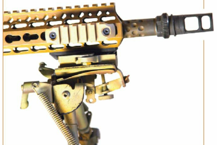
AAC muzzle brake/suppressor mount tops off now-dimpled RPR match barrel.
